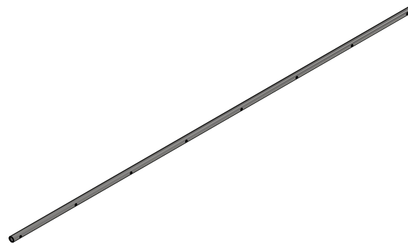
TB2MAA-CUS999-0417 - Round Tubing .12 WALL x 1" O.D. x 87" LG.
