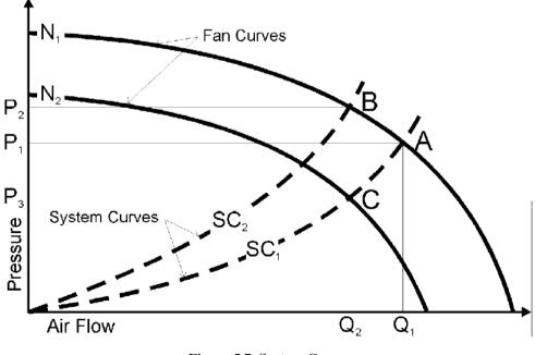
Figure 5.7 System Curve
