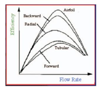
Figure 5.9 Fan Performance Characteristics Based on Fans/ Impellers
