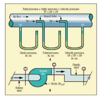
Figure 5.15 Static, Total and Velocity Pressure
