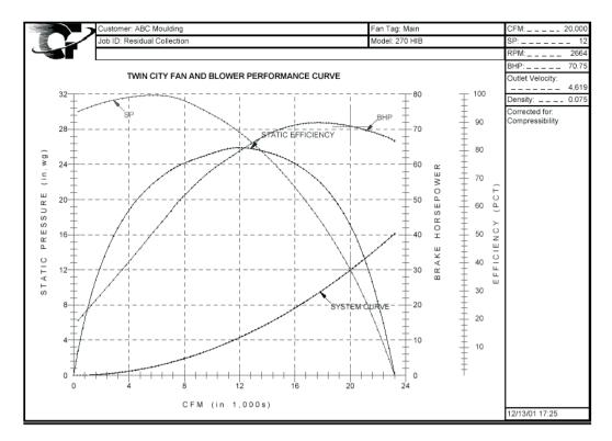
Figure 5.6 Fan Characteristics Curve by Manufacturer
