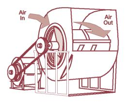
Figure 5.1 Centrifugal Fan
