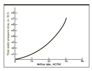
Figure 5.5 System Characteristics
