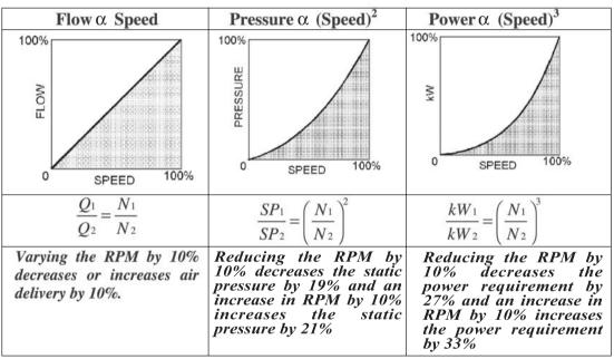
Where Q – flow, SP – Static Pressure, kW – Power and N – speed (RPM)
