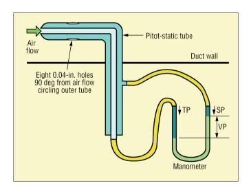
Figure 5.16 Velocity Measurement Using Pitot Tube
