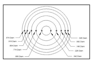
Figure 5.17 Traverse Points for Circular Duct
