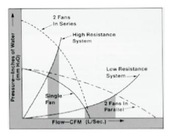
Figure 5.13 Series and Parallel Operation
