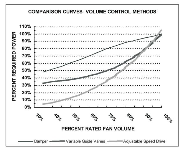
Figure 5.14 Comparison: Various Volume Control Methods
